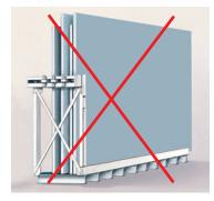
Secure and strap any wall elements for interim storage in the <u>in-loader</u> (for several days).
