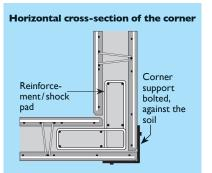
Secure the concrete pressure at the corner and the T-joints, for example the steel brackets, bracing against the soil or bolting a base plate.
