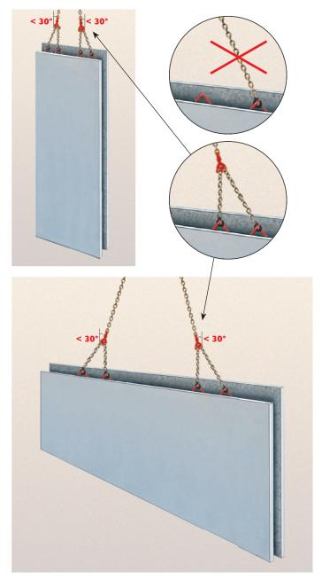
With the supplying factory, coordinate the use of only **2 special lifting links** (heavy walls) with high load-bearing capacities of above 5 tonnes each.
