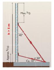
When the wall elements are higher than 5 m (refer to the assembly statics), use the small support in addition to the large one.
