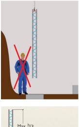
No one is allowed between the wall and the embankment when the crane is in operation and a wall element is being deposited.
