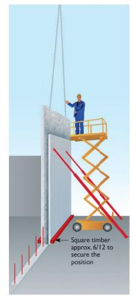
Mount the supports to the element using screws and U-shaped discs. Fasten the supports to the base plate with the approved dowels. Dowels have already been integrated into the wall element at the factory. Refer to the **assembly plan** for further information.
