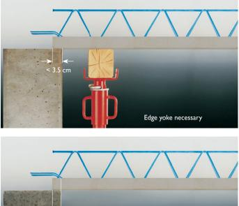
$a \ge 3.5$  cm: n edge yoke is unnecessary if at least every second lattice girder rests on a lower belt knot and the supporting loads do not exceed the values defined in the authorisation.
