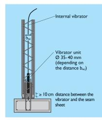
When compacting the concrete, ensure that the internal vibrator does not come into direct contact with the concreted joint seal.
