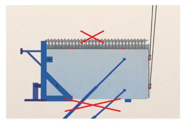
According to accident prevention regulations, special guards to prevent falls are necessary in exceptional cases. This is when assembly supports and thrust reinforcements were already mounted before the walls were fastened.
