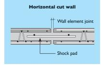
Install the necessary thrust reinforcement and secure the corners according to the statics. As a rule, one strip of shock pad is sufficient.
