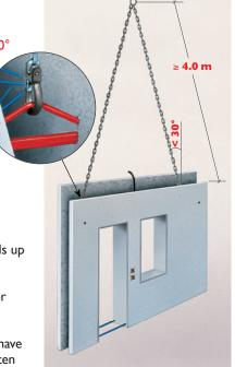
A transport anchor consists of a bracket with cross bolts and is located approx. 25 cm below the top edge of the wall. Cross bolts are made of either round steel, steel pipe or even wood.
