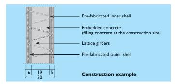
The finished panels (formwork) are 5 to 7 cm thick as a rule. The core concrete must be at least 7 cm thick whereby deviations are possible in exceptional cases. For the wall construction, comply with the authorisation by the building authorities (refer to the assembly plan).
