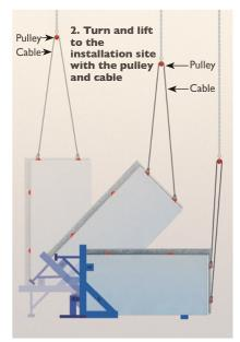
Anchor high walls throughout or secure them with clamps for better joint alignment.
