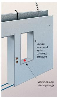
Secure the formwork against concrete pressure in the direction of the wall at the wall ends or at the openings.
