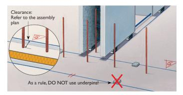
Peculiarities will arise when the floor plan is applied. As a rule, the single-row connecting reinforcements are located approx. 3 cm away from the inner shell.
