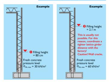
Coordinate with the factory to reduce the distance in the lattice girder. Do not install additional layers of concrete until the preceding layer has set  $t_E$  (period of time for mixing until setting is complete according to DIN).
