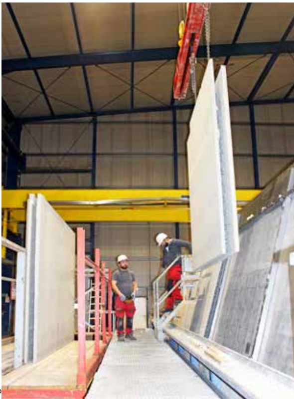
Completely hardened double-wall elements
