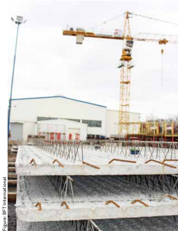
Complete floor elements in the storage yard
