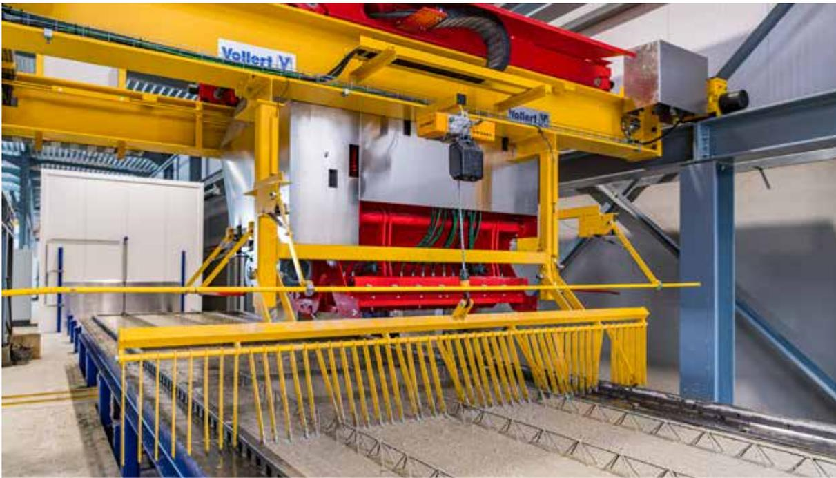
Mechanical roughening of floor slabs using “knives” attached to the concrete spreader that penetrate into the fresh concrete during spreader travel and imprint the ribbed texture
